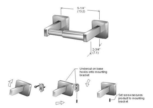
**Mounting of Product:** Screw concealed mounting system: The mounting bracket is attached to the wall with screws at the desired height. The unit is then hooked onto the bracket. When the set screw is tightened the product is firmly secured to the wall. The set screw applies pressure to an inclined surface on the bracket this provides a rattle free and integral mounting of the product. (mounting bracket and screws provided).
